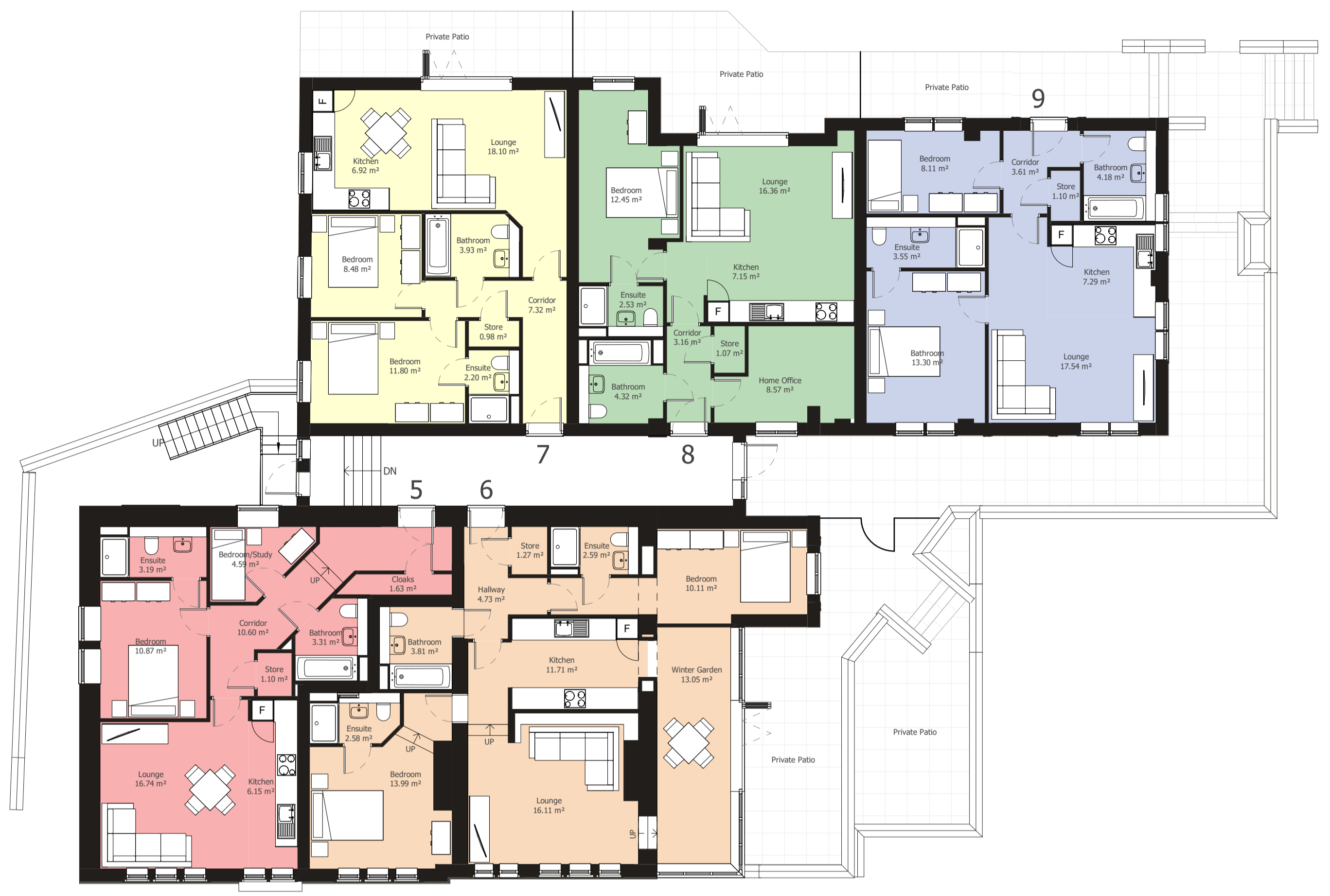
Proposed First Floor Plan 1 : 100
